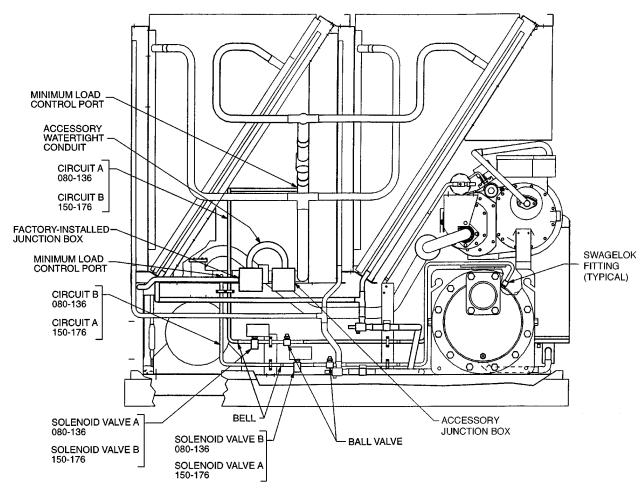
Fig. 3 — Installing Valves, 30GX
